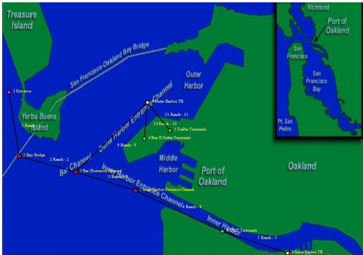
Figure 4-2. Oakland Harbor HarborySym Node Network
